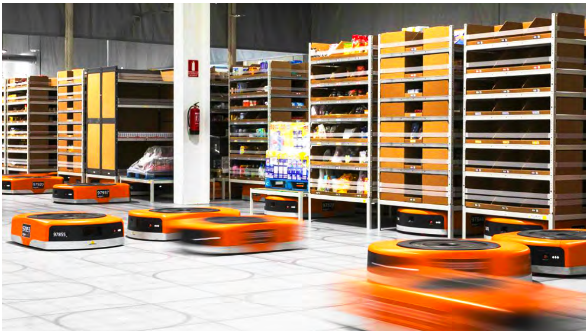
Amazon Robotics develops software and manufactures machinery to automate the flow of inventory in Amazon fulfillment centers. [Source: Amazon]
