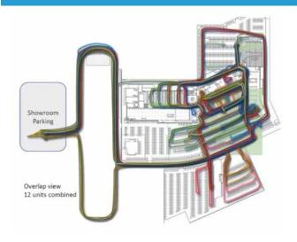
Vehicles were moved more than two miles through multiple staging areas during the reconditioning process prior to creating a new streamlined process.
